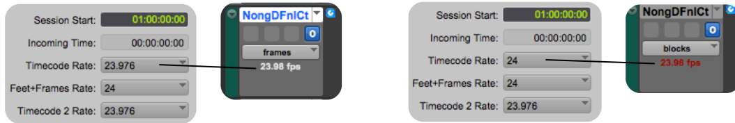
Session Timecode Rate Matches the QuickTime Video (Left) and QuickTime Video Mismatch (Right)
